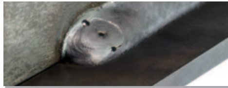
With crater filling – perfect end of weld seam
